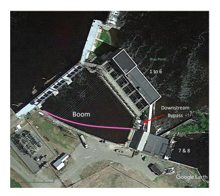
The model assumes effectiveness/guidance of 53% based upon observations at the Lockwood Project. At Lockwood, the boom crosses the power canal upstream of the units. This is not the case at Shawmut where the boom is not upstream of all units. Combined with much lower expected encounters of the boom by smolts, it is incorrect to assume 53% guidance by the boom. As the difference in mortality for the bypass versus units 1 to 6 is nearly 9%, survival results are incorrectly inflated.
