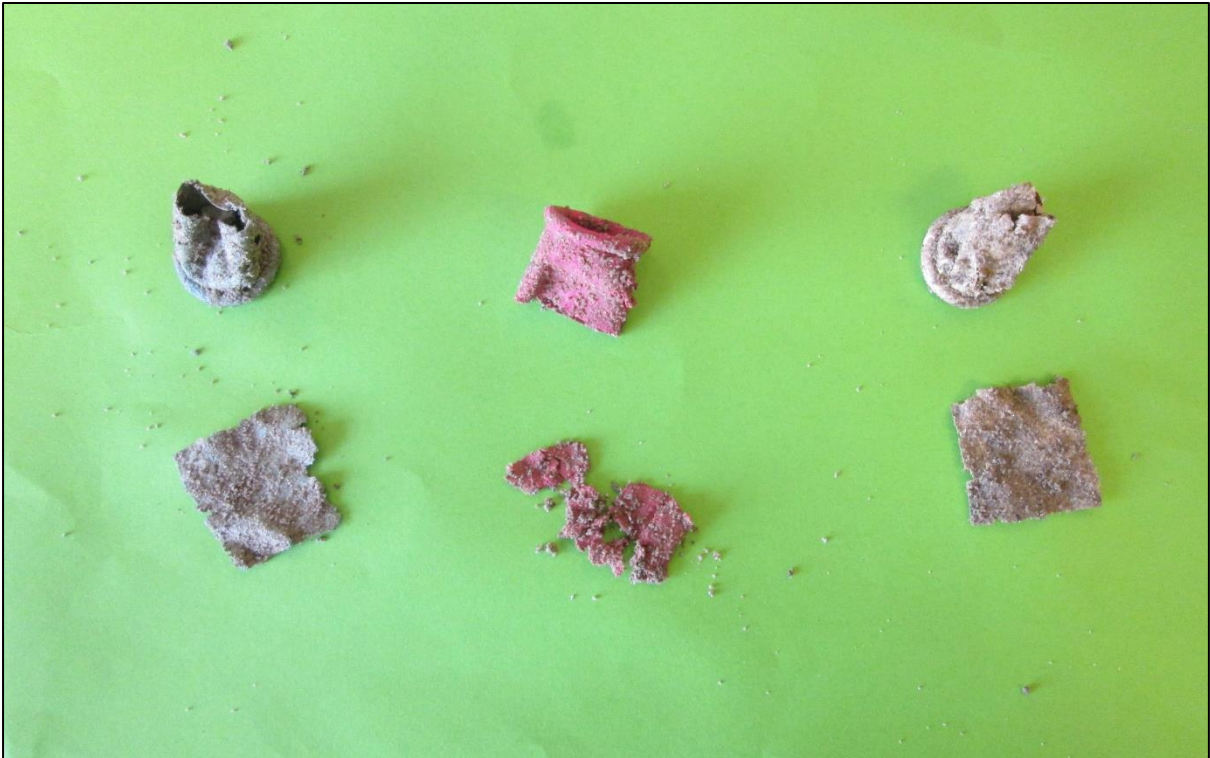
Figure 6. Visual presentation of Balloon after 9 months of incubation in soil
