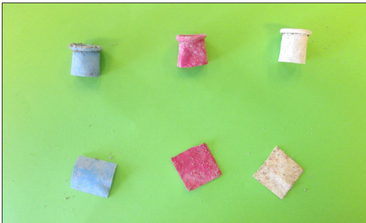
Figure 4. Visual presentation of Balloon after 6 weeks of incubation in soil
