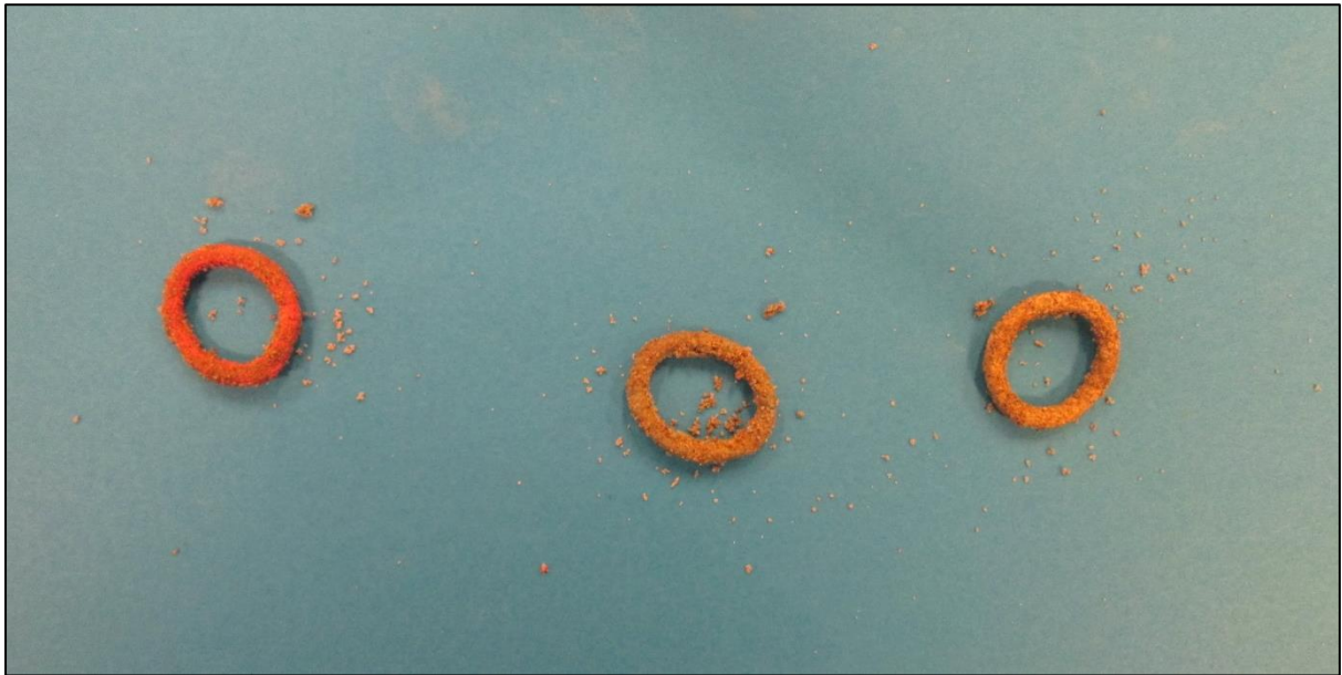
Figure 8. Visual presentation of Balloon after 2 years of incubation in soil
