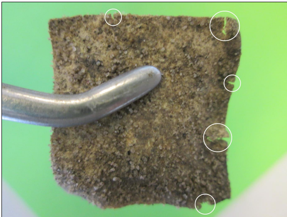
Figure 5. Detailed view of signs of disintegration of Balloon after 6 months of incubation
