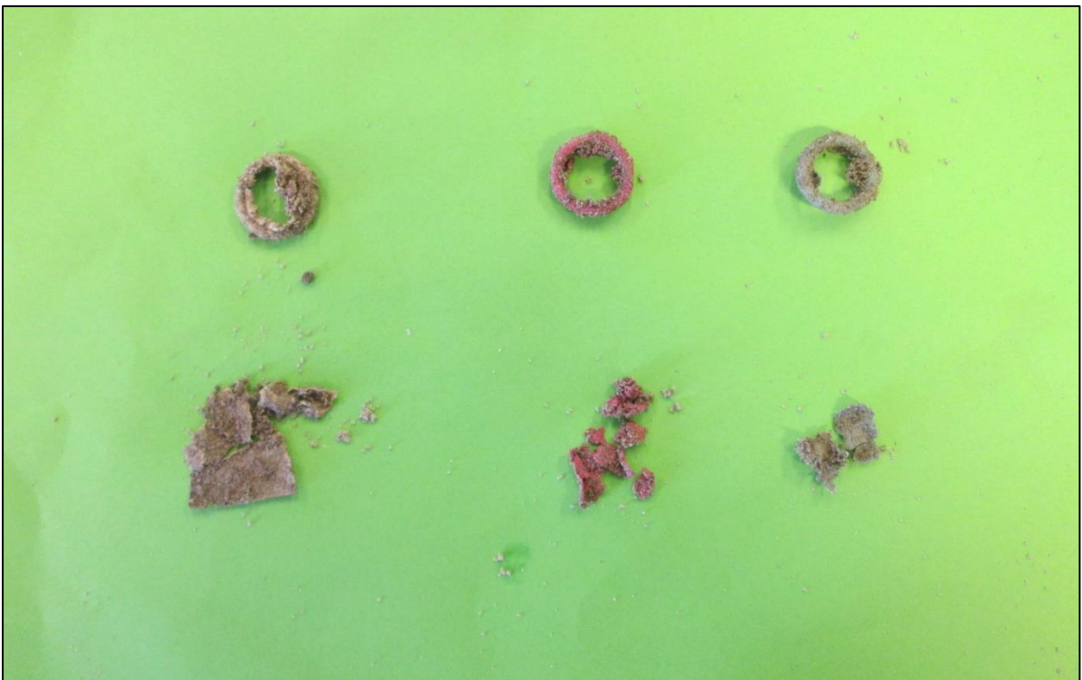
Figure 7. Visual presentation of Balloon after 1 year of incubation in soil
