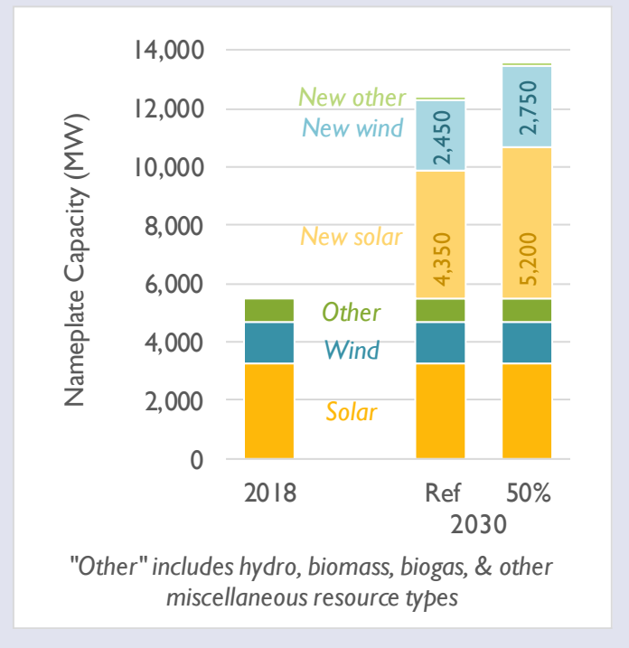
Figure 2. New and incremental renewable capacity additions in the New England electricity system
