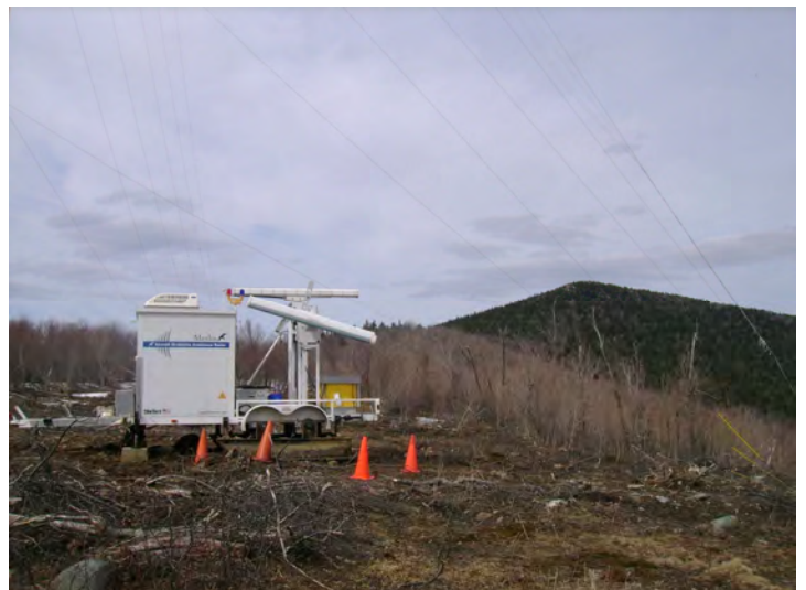
A radar unit on top of the mountain monitors migrating birds 24 hours a day for 30 days in the spring and 30 days in the fall.
