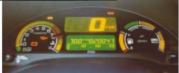
Above: The Insight’s control panel monitors current and lifetime miles per gallon; Brian’s average is 70 mpg.
